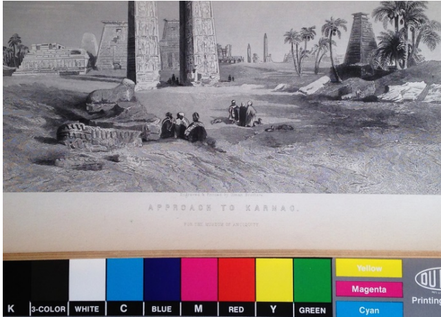
Figure 1: Example of poor usage of an outdated imaging test target
