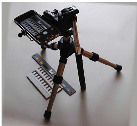
Figure 1: Mobile phone camera used in small copy-stand arrangement
