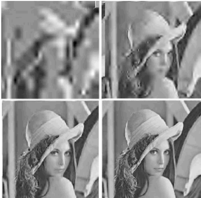
Fig. 1. Reconstructed image after decoding bit-planes 2, 4, 6, and 8 (from Ref. 1)
