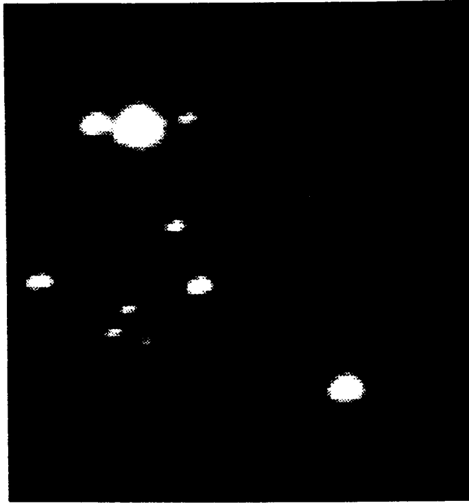
Figure 6: Upper Image is the initial 600 second image of a star field taken through a Z filter. Lower image is the following 600 second dark exposure (shutter closed) showing residual images at location of saturated stars seen in upper image. The images are the result of a 4x4 block average of 484 x 524 physical pixels.
